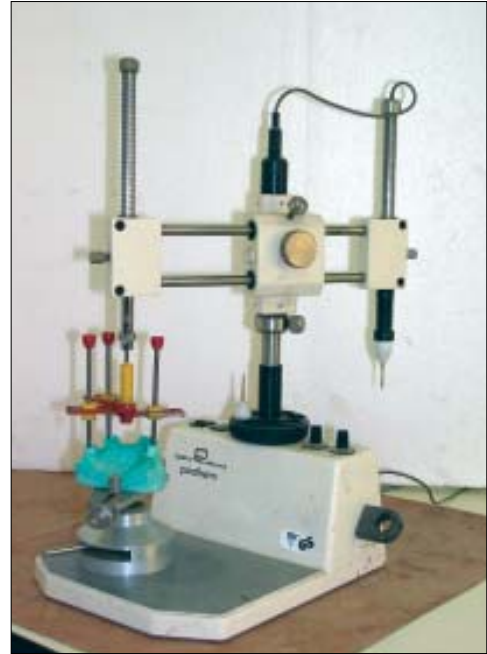
Figure 3: The Tripoder attachment mounted on surveyor and positioned on cast
