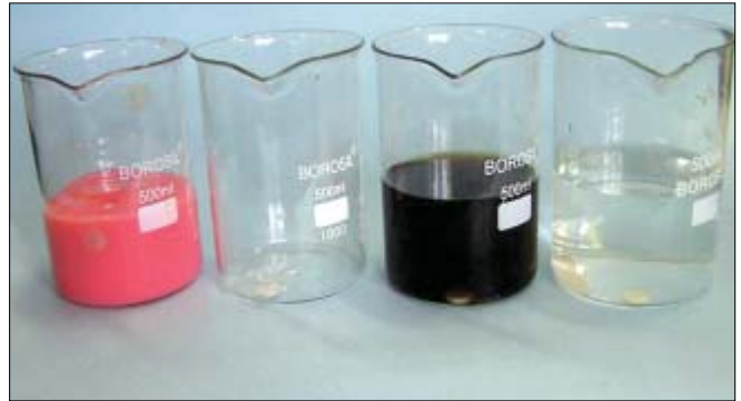
Figure 4: Ceramic specimens immersed in 1.23% APF Gel, 16% Carbamide peroxide, Coca-cola and distilled water
