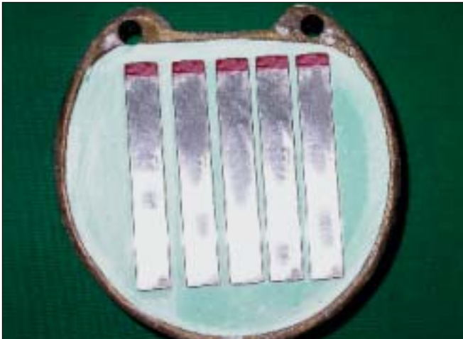
Figure 2: Preformed dies invested in dental stone for preparation of samples for transverse strength
