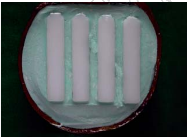
Figure 3: Preformed plastic strips invested in dental stone for preparation of samples for Impact strength
