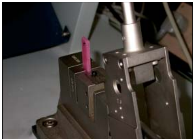
Figure 6: RESIL Impact tester (Izod test)
