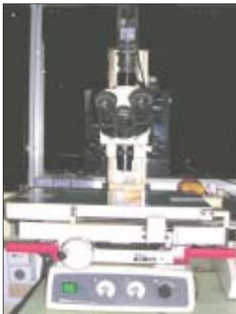
Figure 2: Measuring marginal discrepancy using Nikon measurescope
