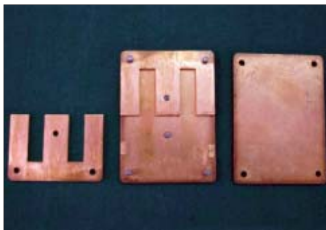
Figure 2: Showing brass mold for standardization of sample size (10 x 50 x 2mm)
