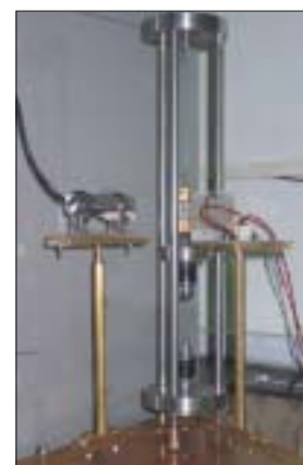
Figure 7: Dynamic visco-elastometer (Torsional Pendulum Apparatus) with laser measuring device
