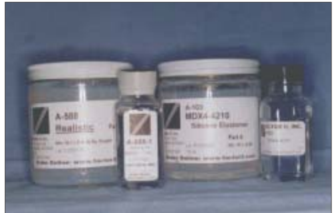
Figure 3: Maxillofacial silicone test material: A-588V-1, MDX 4-4210
