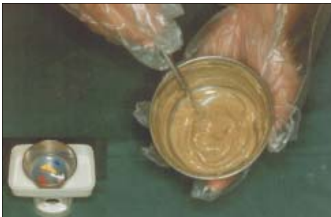
Figure 4: Proportioning and manipulation of parts of silicone elastomer
