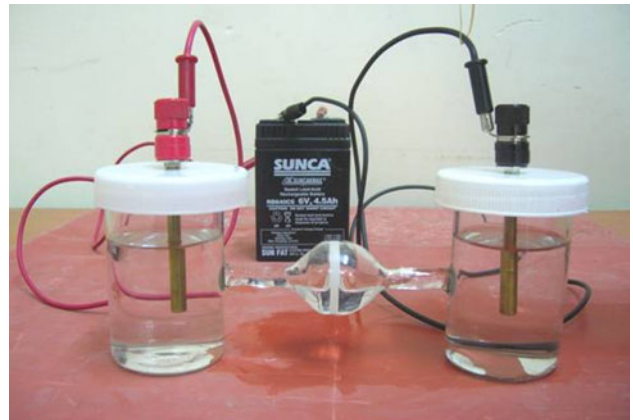
Fig. 2 Custom made electrolyzing apparatus
