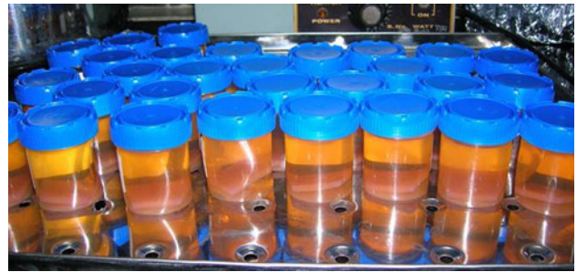
Fig. 1 Heat polymerized acrylic specimens immersed in 50 ml of bacteria suspended solutions
