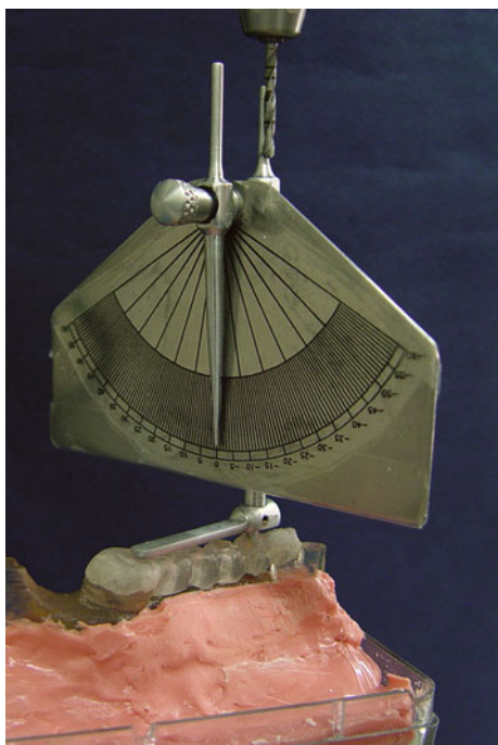
Fig. 6 The horizontal bar was aligned with the central fossa, fixed perpendicular bar was inserted in the milling machine
