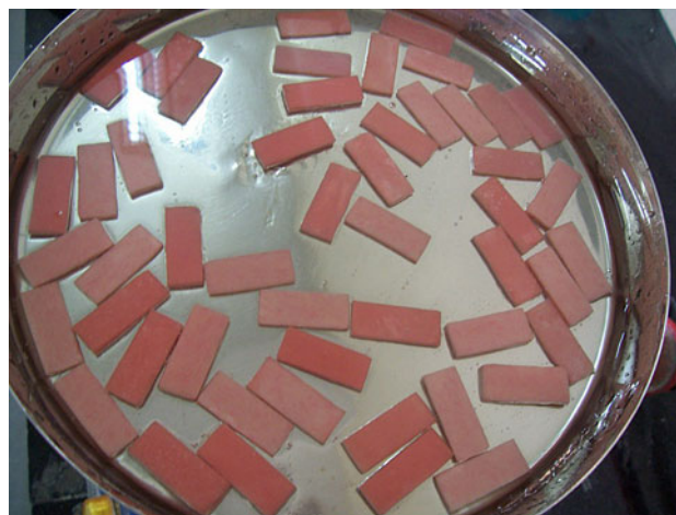
Fig. 2 Experimental specimens immersed in artificial saliva
