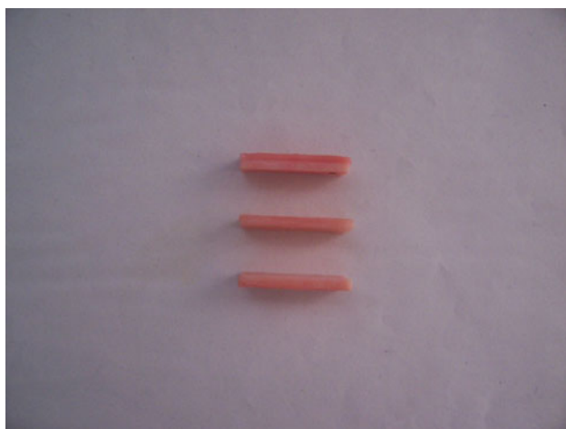
Fig. 1 Acrylic specimens with soft liner material bonded to them
