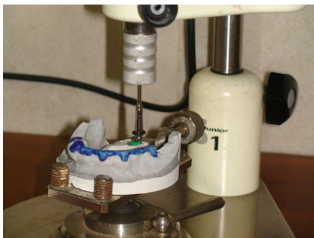
Fig. 11 positioning of castable attachments with milling machine
