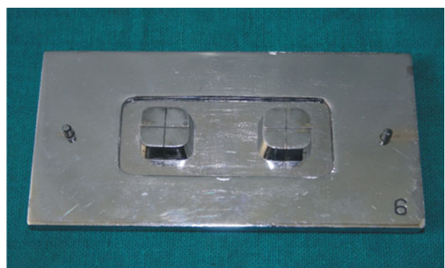
Fig. 4 Master die with guide plate for 6 mm spaced tray
