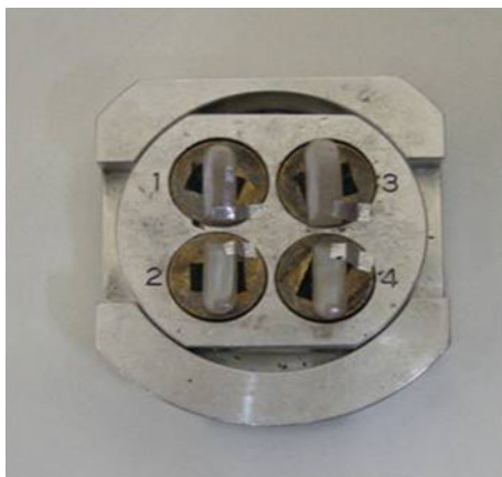
Fig. 7 Four specimens mounted on the mounting plate
