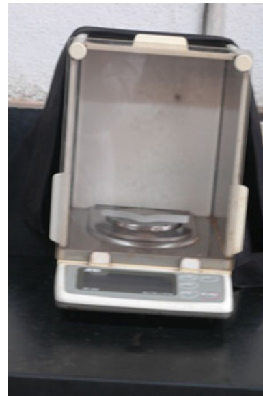
Fig. 6 Test specimen weighed before water sorption
