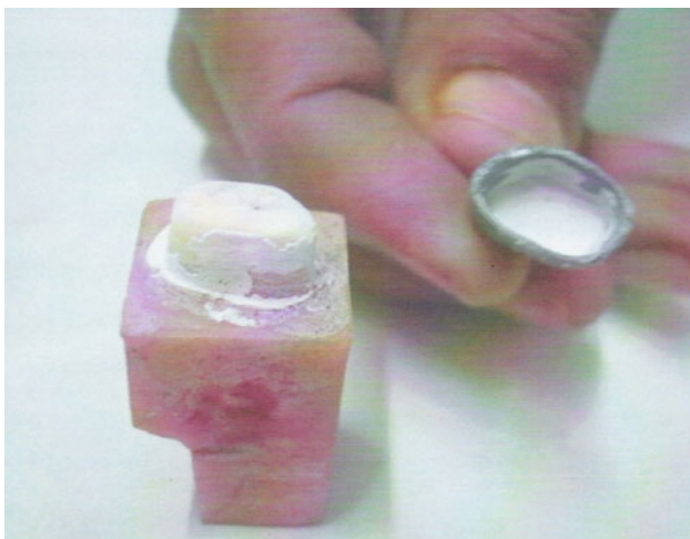
Fig. 3 Zinc phosphate cement without resin sealer showing mixed mode of failure
