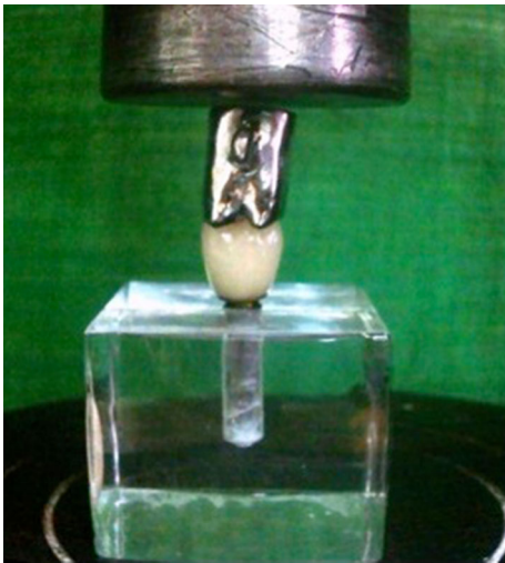
Fig. 4 Vertical static loading applied on the crown cemented on the abutment
