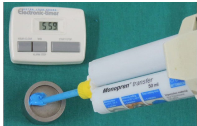
Fig. 5 Application of impression material onto die surface (dry condition)
