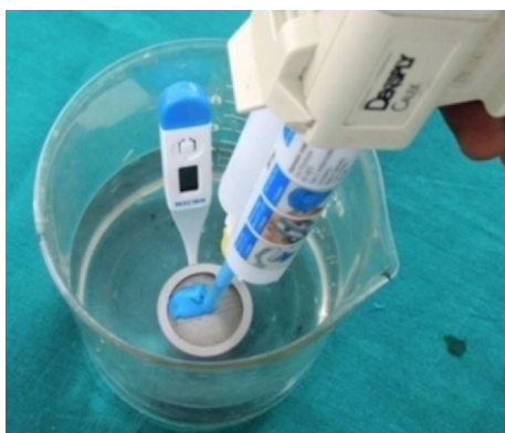
Fig. 7 Preparation of sample under wet condition
