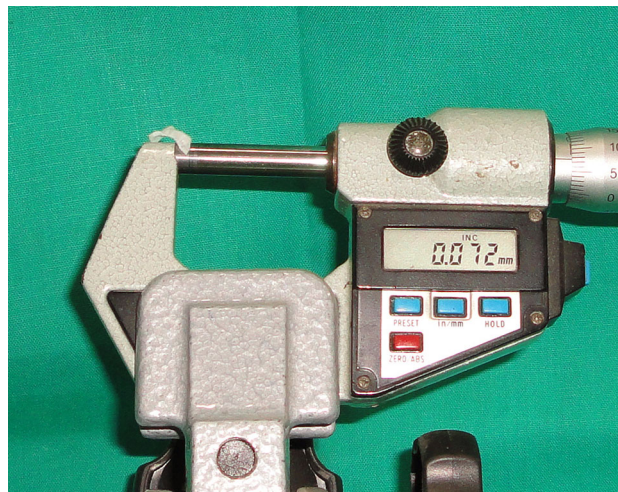
Fig. 5 Measurement of PCS with micrometer
