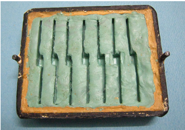
Fig. 4 Removal of the spacers and the processed specimens from the flask
