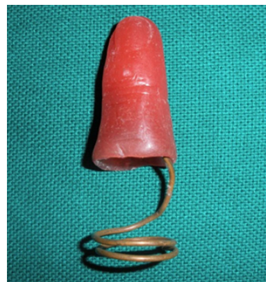
Fig. 3 Wax pattern with copper wire
