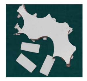
Fig. 2 Commercially available pre sintered zirconia
