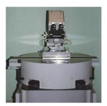
Fig. 3 Measuring microscope (Resolution 1 µm)
