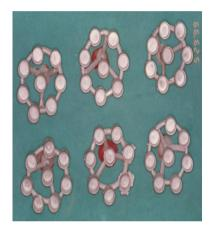
Fig. 6 Metal frameworks showing various groups of castings
