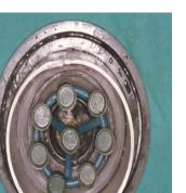
Fig. 5 Wax patterns before investing attached to sprue former
