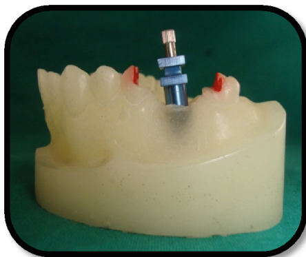
Fig. 3 Different groups of impression technique (a) Group I: Non modified square impression coping (b) Group II: Adhesive coated square impression coping (c) Group III: Sand blasted square impression coping (d) Group IV: Sand blasted and adhesive coated square impression coping
