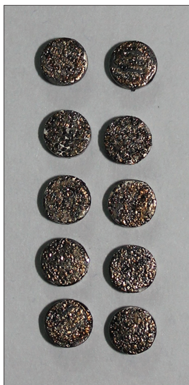
Figure 2: Laser surface-modified and conditioned titanium zirconium samples
