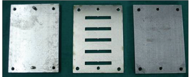
Figure 2: Three-piece stainless steel metal mold for impact strength specimen five rectangular cavities (50 mm × 6 mm × 4 mm) in the middle part
