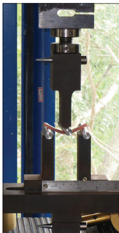
Figure 5: Specimen subjected to flexural strength testing under three-point loading
