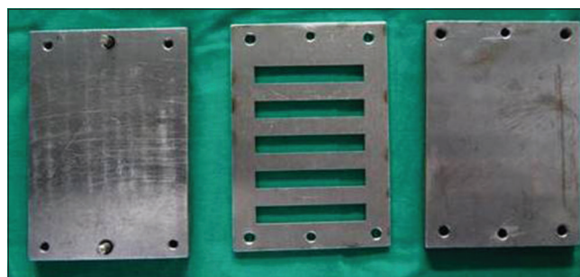
Figure 1: Three-piece stainless steel metal mold having five rectangular cavities of dimensions 64 mm × 10 mm × 3.3 mm in the middle part
