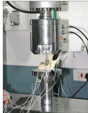
Figure 7: Load application on the crowns using universal testing machine
