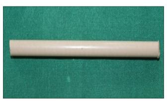
Figure 1: Poly-ether-ether-ketone ingot before milling
