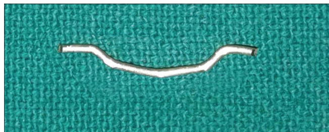
Figure 4: Stainless steel wire configuration with straight ends
