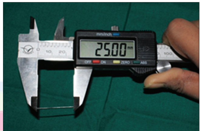
Figure 3: Crosschecking length of casting using digital vernier Caliper
