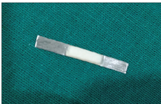
Figure 6: Porcelain buildup on castings
