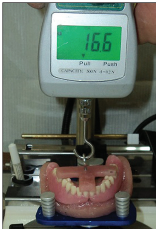
Figure 3: Retention measured with digital force gauge (original photograph)
