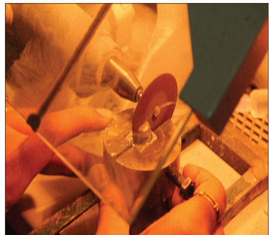
Figure 9: Sectioning of samples
