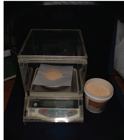
Figure 4: Electronic measuring balance used for weighing dental stone
