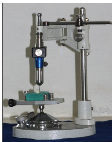
Figure 1: Tooth positioned on cast holder on surveyor and handpiece attached to the surveying arm
