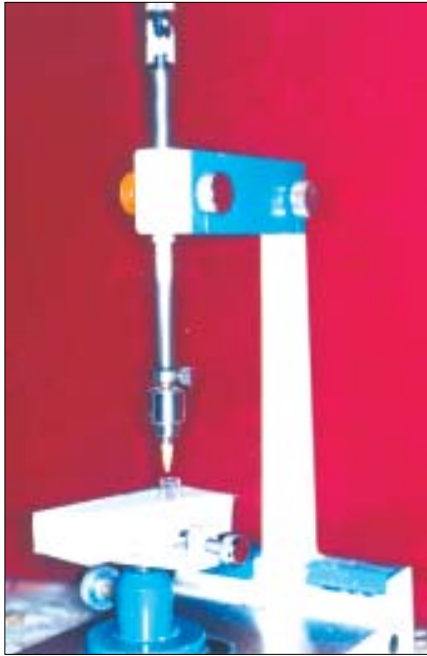
Figure 6: Dental surveyor used to mount teeth in plastic cylinder
