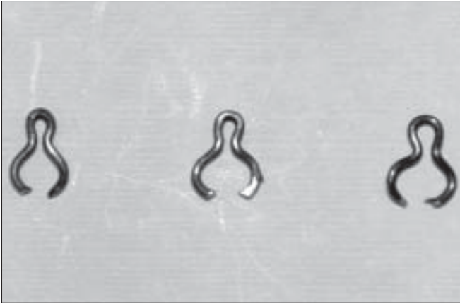
Figure 8: Clips collapsed to different sizes based on the diameter of the bar
