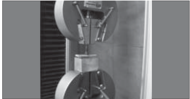
Figure 4: Flexural strength testing on Universal Instron testing machine
