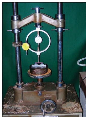
Figure 4: Tri-axial loading frame for testing transverse strength
