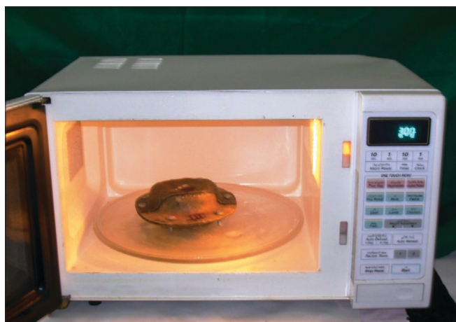
Figure 2: Microwave oven with fibre flasks
