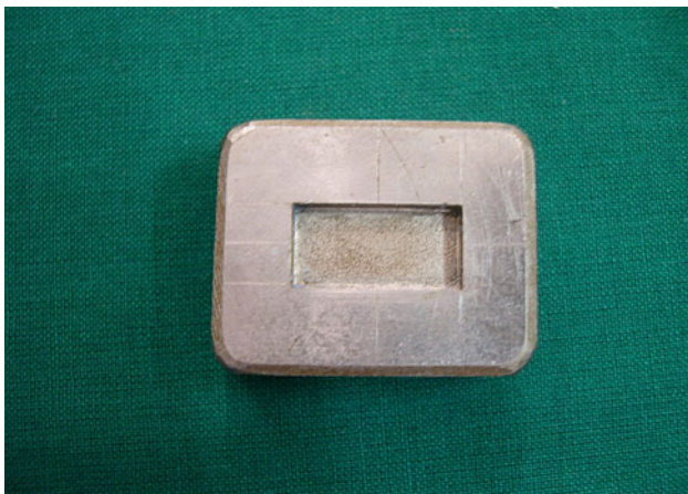
Fig. 2 Master die used for making rectangular wax patterns
