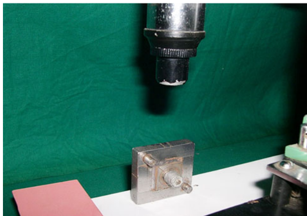
Fig. 3 Evaluation of crown casting for marginal discrepancy under Travelling microscope
