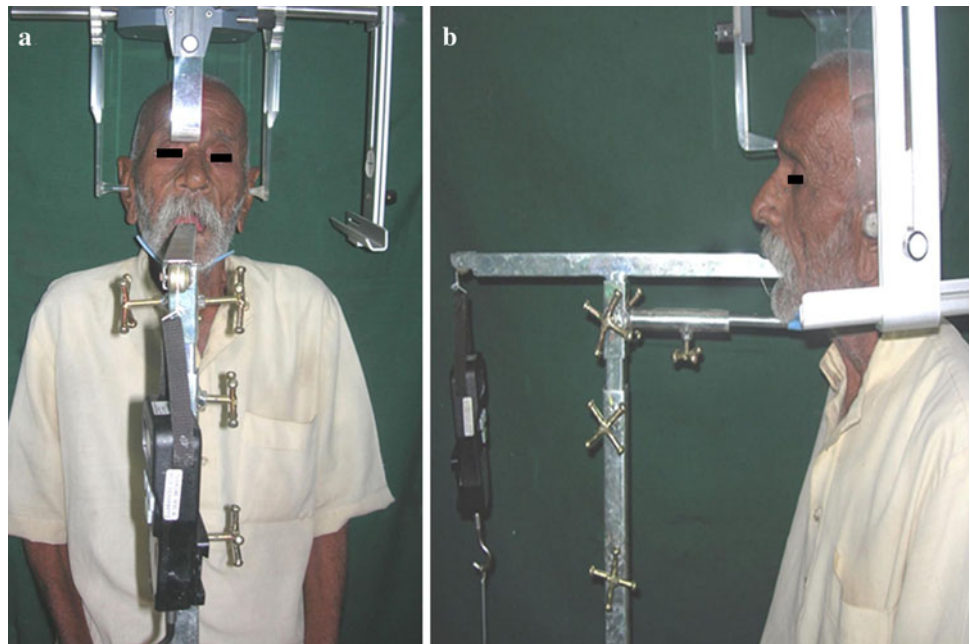
Fig. 6 Measuring of retentive force using the specially designed apparatus & cephalostat. a Frontal view. b Profile view
