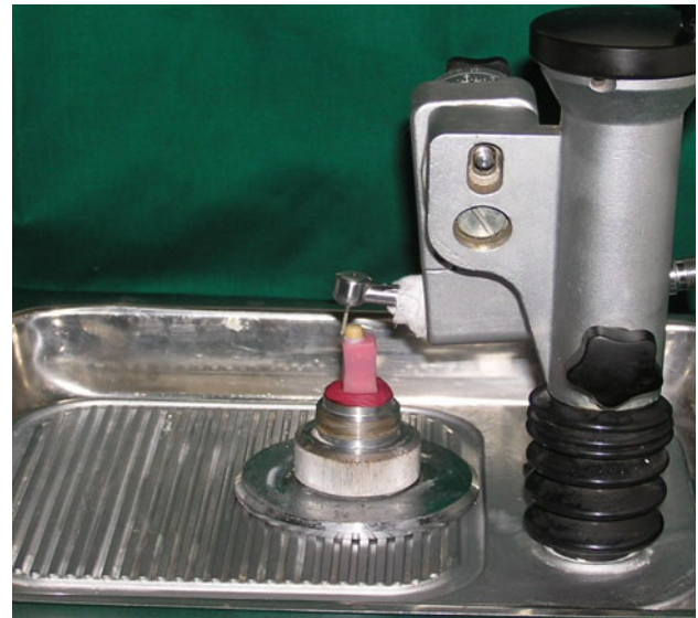
Fig. 3 Specimen with high turbine hand piece mounted in K-9 crown finishing installation
