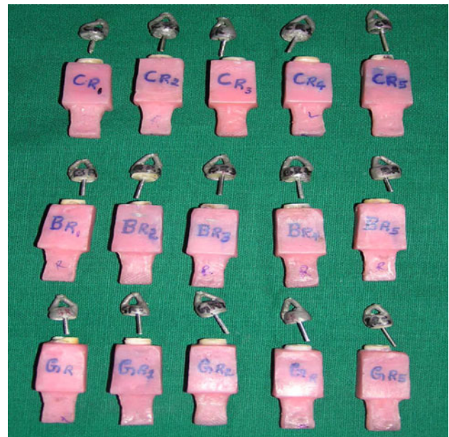
Fig. 5 Debonded specimens with post, core and cast crown
