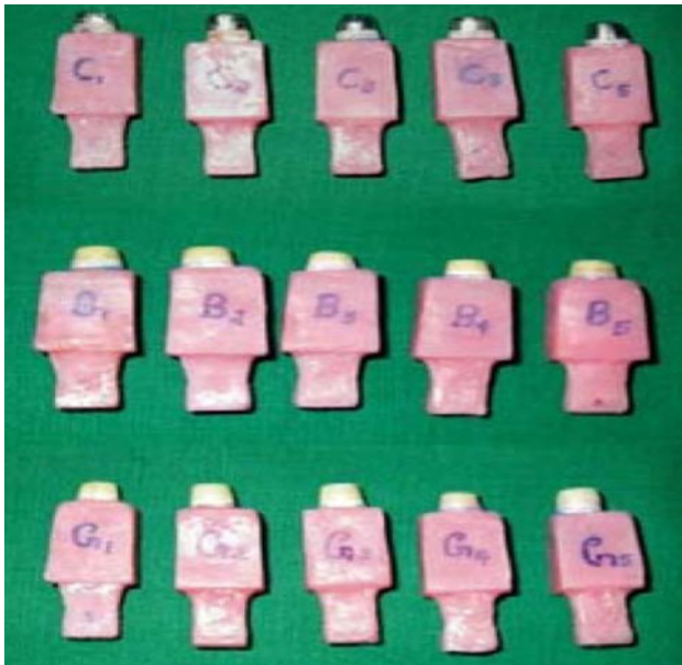
Fig. 2 Prepared cast core, composite core and glass ionomer core specimens
