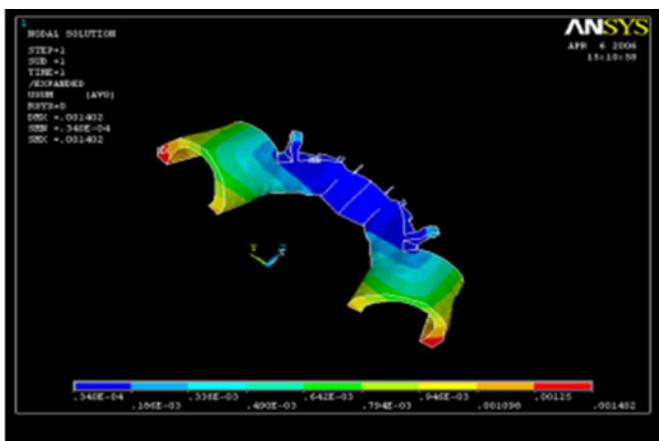
**Fig. 13** Displacement among different parts of lingual bar and lingual plate in Kennedy’s Class I situation under applied load
