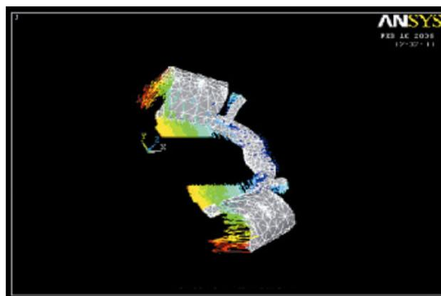
**Fig. 8** Application of load to the cast partial denture framework
