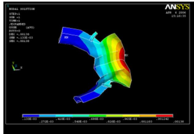
**Fig. 16** Displacement among different parts of lingual bar and lingual plate in Kennedy's Class IV situation under applied load
