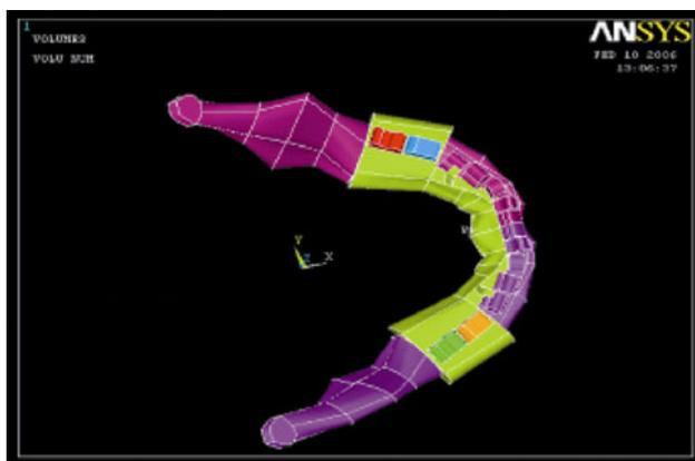
**Fig. 7** Solid volume finite element of the entire dentulous mandible and cast partial denture framework
