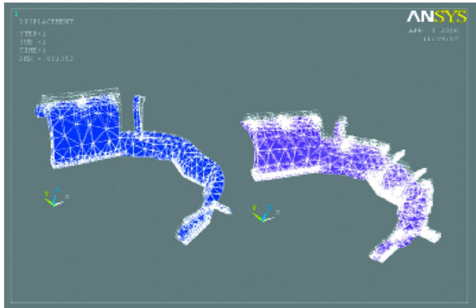
**Fig. 11** Maximum displacement among Class III lingual bar and lingual plate Kennedy's situation under applied load
