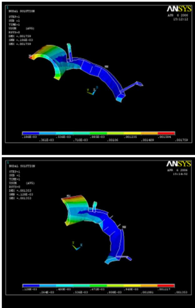
**Fig. 14** Displacement among different parts of lingual bar and lingual plate in Kennedy's Class II situation under applied load
