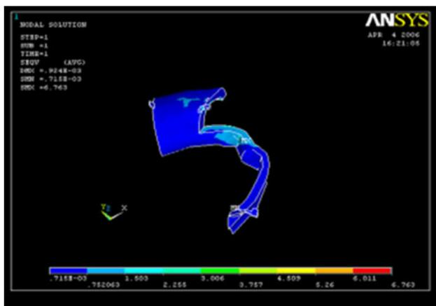
**Fig. 15** Displacement among different parts of lingual bar and lingual plate in Kennedy's Class III situation under applied load
