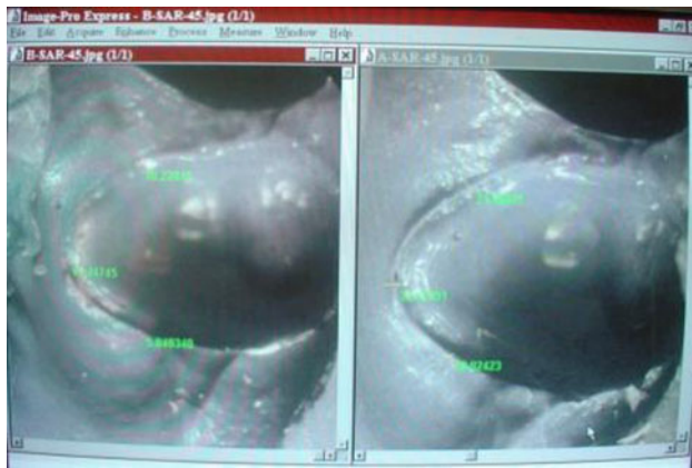
Fig. 8 Stereomicroscopic and image-analysis of impressions made before retraction and after retraction to measure horizontal retraction (in one-tenth of microns)
