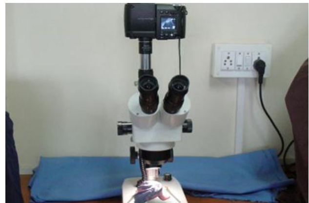
Fig. 2 Stereomicroscope used to measure horizontal gingival retraction
