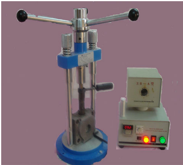
Fig. 3 Flexible injection system
