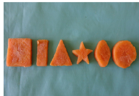
Fig. 3 Test pieces of six forms of square, rectangle, triangle, star, oval, circle—5 mm thick, 10 mm diameter
