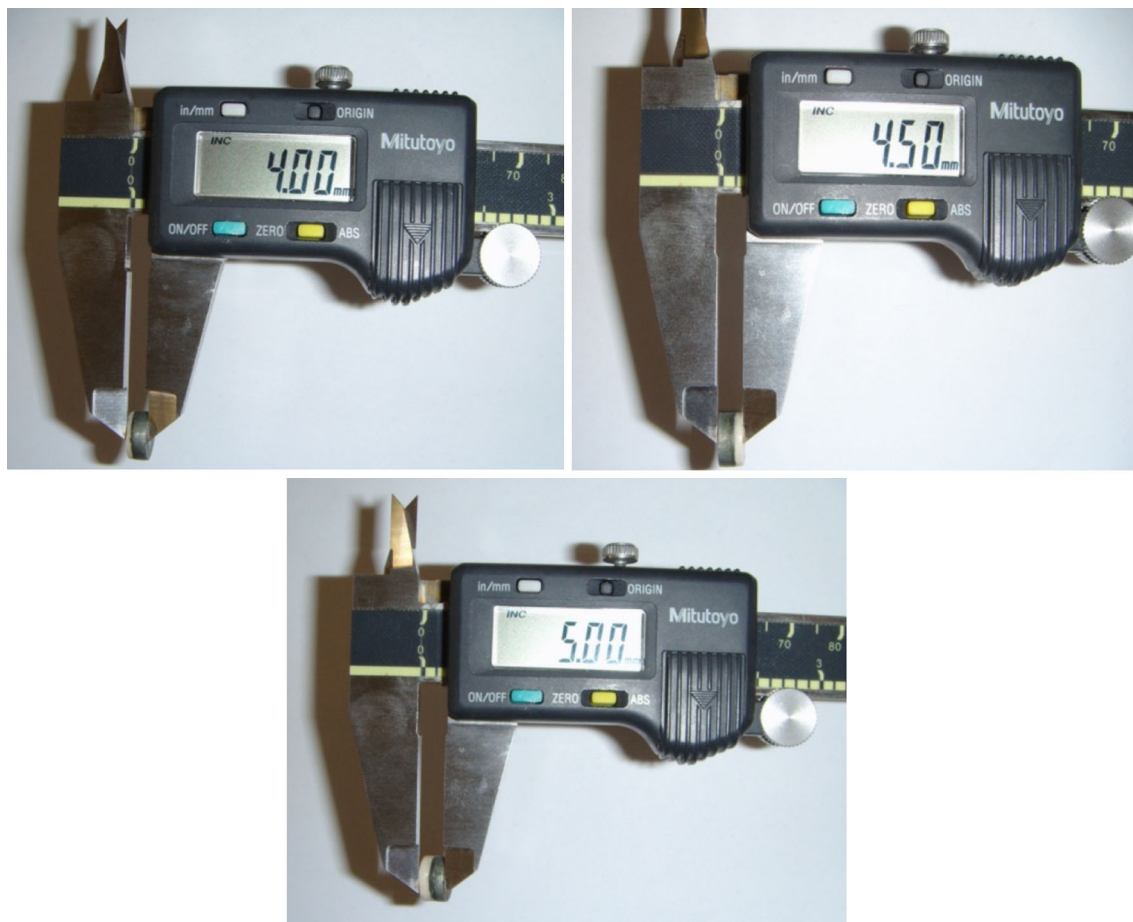
Fig. 3 Digital vernier caliper used to measure thickness of the three groups of samples
