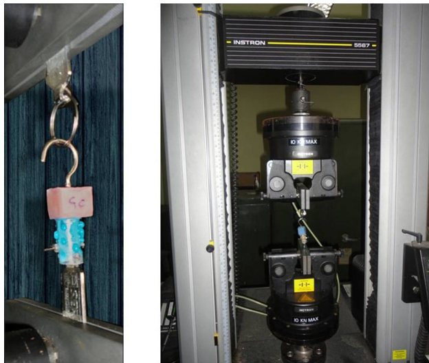
Fig. 4 Sample placed within the Instron machine
