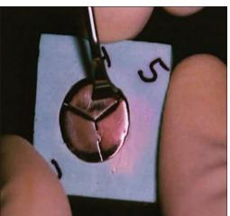
Figure 1: Hand scaling on the representative division of the specimen
