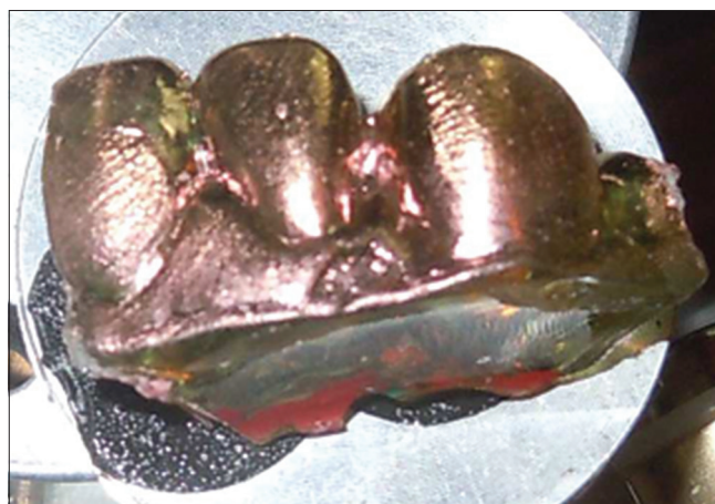
Figure 2: Gold sputtered epoxy resin dies
