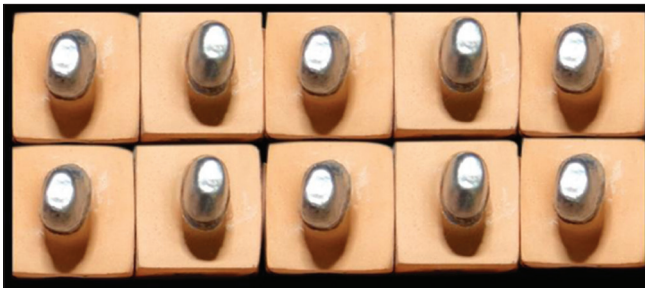
Figure 5: Titanium copings without surface treatment
