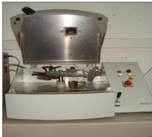
Figure 5: Casting machine (Bego, Bremen, Fornex T)
