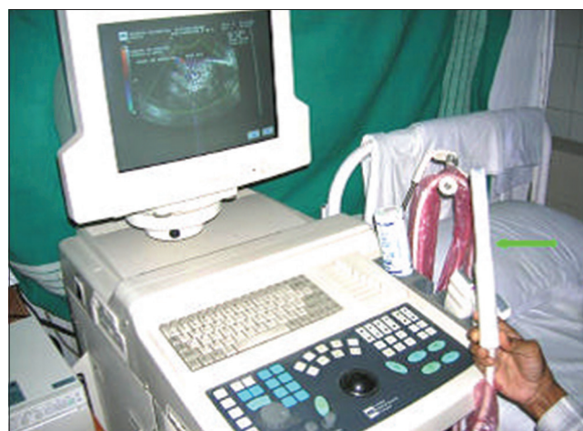
Figure 1: HDI 1500 – ATL unit with three-dimensional and color Doppler facilities (green colour marked is intracavity transducer probe)
